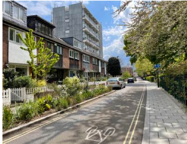
Planting to help narrow the carriageway and calm traffic.
